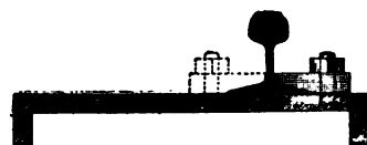
FIG. 156.—CROSS-SECTION OF RAIL-FASTENING.
