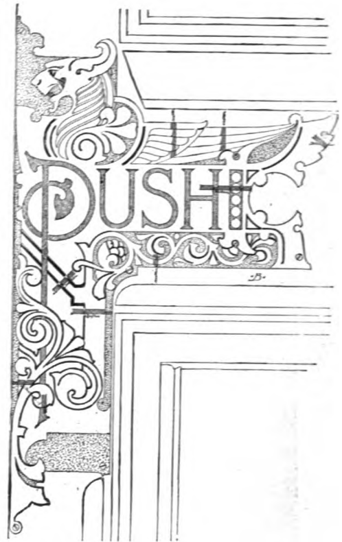
FIG. 639.—DETAIL OF PUSH-PLATES OF DOORS.
