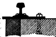
FIG. 145.—CROSS-SECTION OF RAIL-FASTENING.
